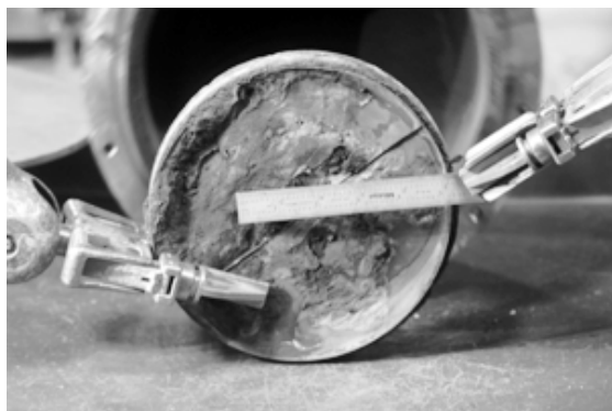
Fig. 1. Metal waste form ingot prepared from irradiated EBR-II cladding hulls.
